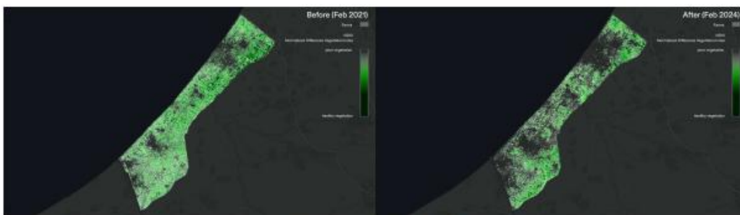
Figure 6. NDVI analysis shows areas covered with vegetation. Map (left) shows plant life in Gaza in February 2021, and map (right) shows plant life in February 2024. Cloud free mosaics of Sentinel-2 satellite data between 20 January and 8 February of 2021 and 2024 is used as the bases of this NDVI study. (Forensic Architecture)
